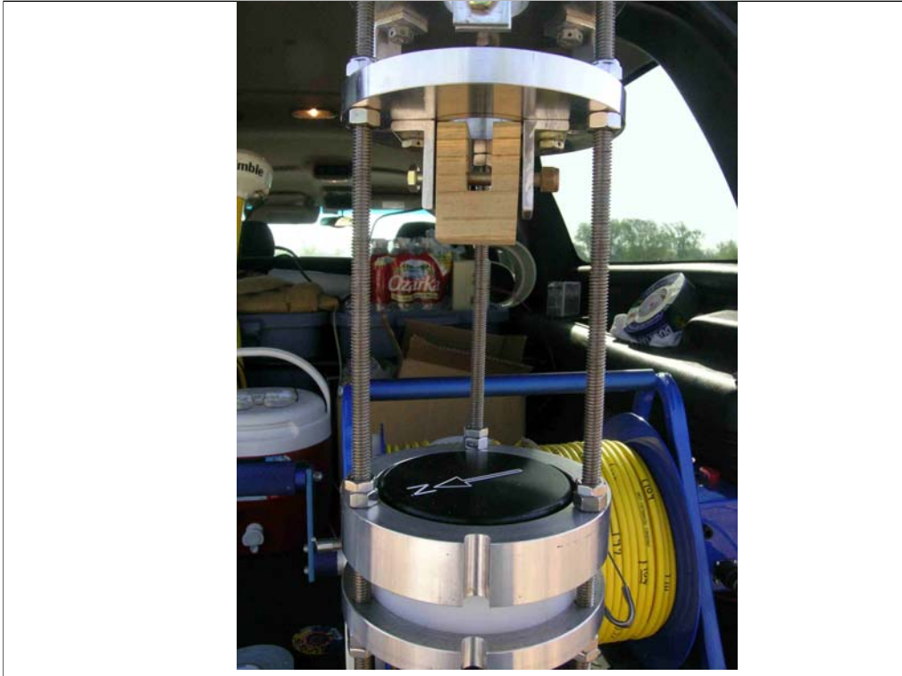
Point of attachment of the cable to the sonar tool's framework. The stainless steel loop of the cable-support grip is inserted into the notch in the wooden block and secured with the bolt.
